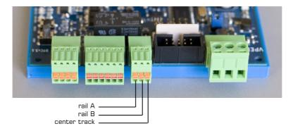
The DTCv3 can reverse the polarity of the track on the bridge to ensure it is identical to the polarity of the exits. Rail A and B are interchanged between J6 and J7 when polarity is reversed.
