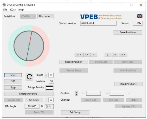
You can rotate the bridge with the arrow-buttons <<<<<<>>> and >>>. More arrows is faster<sup>4</sup>. It actually shows itself. Press and hold as long as you want to turn. To "lock" a button, click on it and drag it away while holding down the mouse button. For some reason, that trick doesn't work on a Mac. Unfortunately for now, a solution has yet to be devised.
