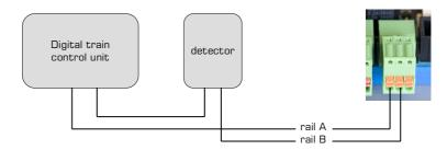
When using a Dinamo system you use a free block output of a TM44 or TM H+CD16. The A terminal to pin 1, one of the B terminals to pin 2.
