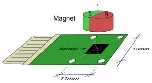
Connecting the DTx sensor to the DTCv3 is easy. Plug one end of the supplied cable into the sensor board and the other end into J10 of the DTCv3.
