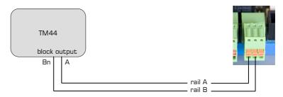
With 3-rail you connect the connection for the center rail of your digital system to pin 3. The connection for the rails of your digital system goes to pin 1 and the same connection for the rails goes to pin 2 via an occupancy detector.
