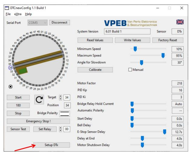
Click "Setup DTx" at the bottom of the window. The right half of the screen and the appearance of the turntable change. The bridge is now a line, consisting of a green and a red half and around the circumference of the turntable a colored border has appeared, half green and the other half red.
