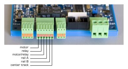
Attention DTCv1 and DTCv2 users: Connections 2 and 3 are reversed on the DTCv3 with respect to the DTCv1/DTCv2.
