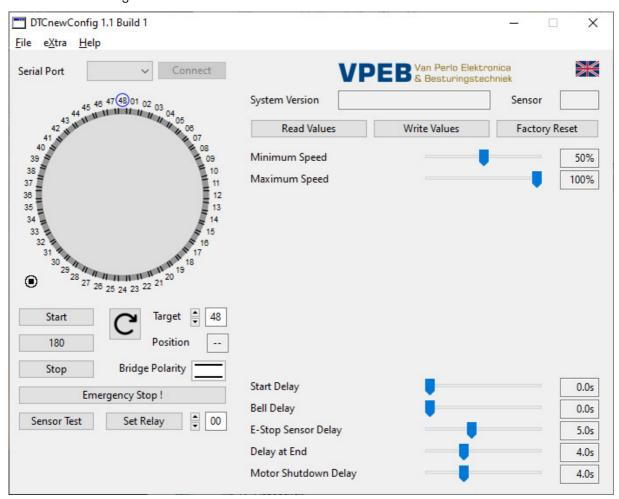
Make sure the DTS, DTZ or DTx sensor is connected to the DTC and turn on the power supply to the DTC. **NOTE**: This order is important because the DTC tests what type of sensor it has at startup. Optionally, you can force a restart by pressing the RESET button.
